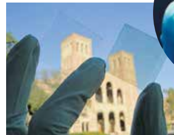
Materials Science and Engineering Professor Yang Yang has developed see-through solar film that could be placed on windows, sunroofs, smartphone displays and other surfaces to harvest solar energy.
